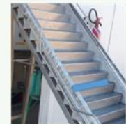
Inorganic coating with photocatalytic material in all steps of the cascade reactor.
